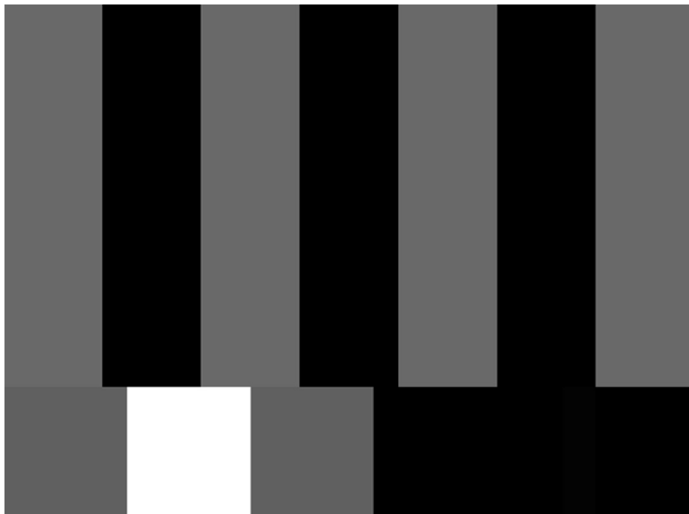
Figure 3. Blue color bars. Caption—On a properly calibrated monitor, blue-only color bars will appear as alternating shades of equal intensity.
