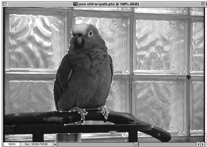
Figure 18.15 We can use Photoshop's Pen tool to outline the bird, and then convert this path to a selection. Because paths are easily modified, it will be easier to change this selection for later frames.
